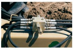
Optional cushion valve protects cylinders and blade components during extreme impacts. For use on RBT40 & 45 Models.
